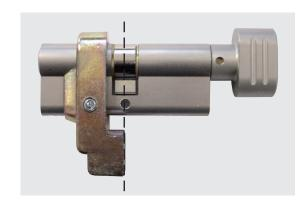
Align the lower part of the Armorshield  $^{\text{TM}}$  with the centre of the cam or screw hole and equally tighten the two grub screws onto the cylinder.
